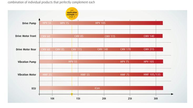
Even, jolt-free starting, driving and rolling set all Linde drive units apart. The key feature of the drive unit in the compactor in this example is the hydraulic traction control. The compactor boasts two hydraulic motors connected in parallel. One of these drives the rear axle, while another rotates the drum.
