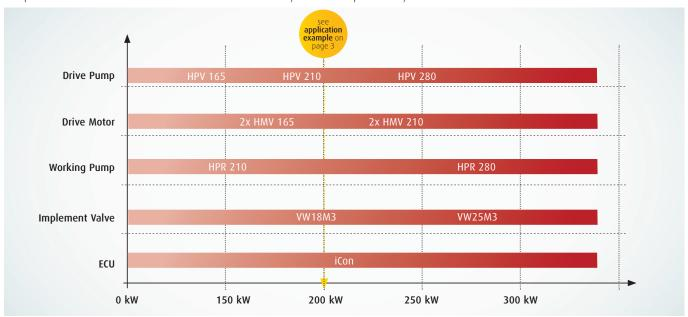
Benefitting from Linde Hydraulics, modern, mobile wood-processing machines are both efficient and sustainable. The example design depicts a wheel-driven wood harvester with two high-performance yet compact hydraulic motors in a closed circuit. This design allows the machine to move safely and protect the soil, even on rough terrain.
